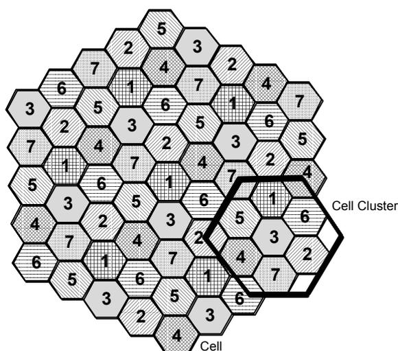
Frequencies cannot be re-used in adjacent cells because of problems with co-channel interference but they can be repeated throughout the network following a pre-set frequency re-use pattern (Figure 3.2).
