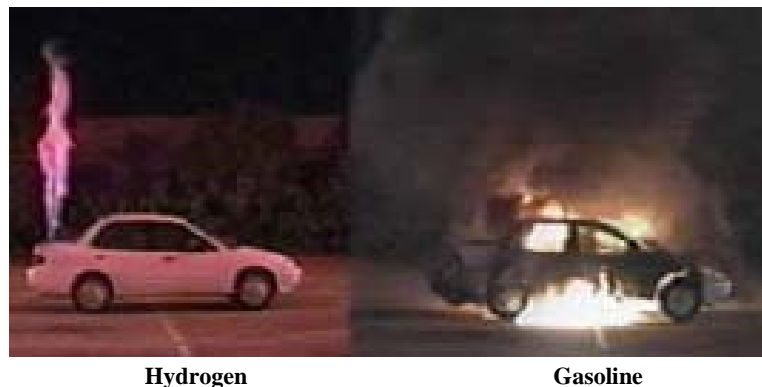
Figure A.12. Hydrogen and gasoline cars 60 seconds after ignition
