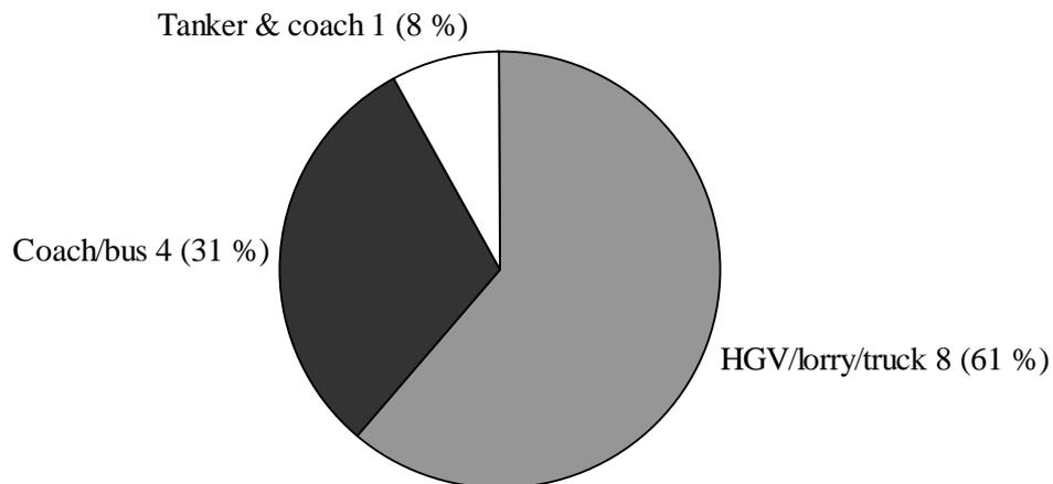
Figure 3: Road Tunnels: numbers of fatalities in fires world-wide (1987-2006), by vehicle involvement. Total = 96 (Not inc. during construction or malicious)
