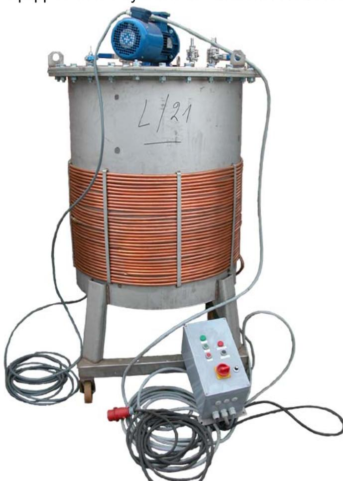
Custom-made reaction vessel with a capacity of 900 litres
